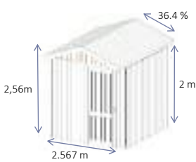
2 pentes shingle et bac acier 36.4%
